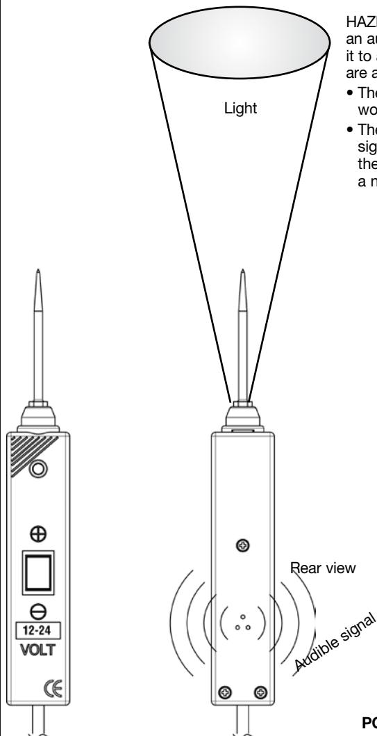
HAZET 2152-5 is equipped with an optical and an audible signal function. After connecting it to a battery, the optical and audible signals are activated.
